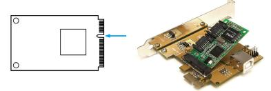
2. Once the mini PCle card is fully inserted into the slot, push the card back against the adapter board. Fasten the mini PCle card to the board with the small mounting screws provided. Make sure not to over-tighten the screws, or you may damage the mini PCle card.
